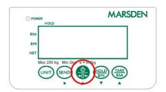
Hold the ON/ZERO/OFF button for three seconds when the scale is turned on. The scale will power down.
