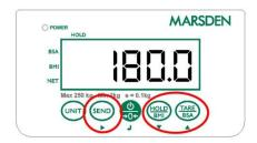
Enter the height by using the TARE/BSA button to decrease the value and HOLD/BMI button to increase the value. To move to the next digit, press SEND.
