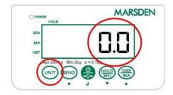
Press the Unit button. The display will change between showing the weight reading in kg/g and in st/lb.
