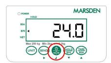
To confirm the height hold down the ON/ZERO/OFF button, after a few seconds the display will alternate between weight, height and BMI.
